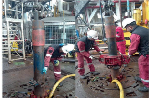
Figure 08-Transfer procedure of SSTT with rig equipment- The 7 5-8 elevators are closed around the pup joint and sit on the dog collar
