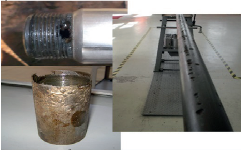
Pump shop findings – Corrosion impact on standard pump metallurgies
