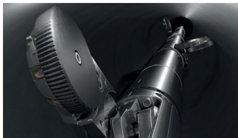
Figure 5: Wheeled drive tractor with three drives seen inside tubing.
