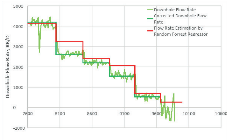
Actual flow rate data and data obtained from low-choke temperature by random forest regression comparison.
