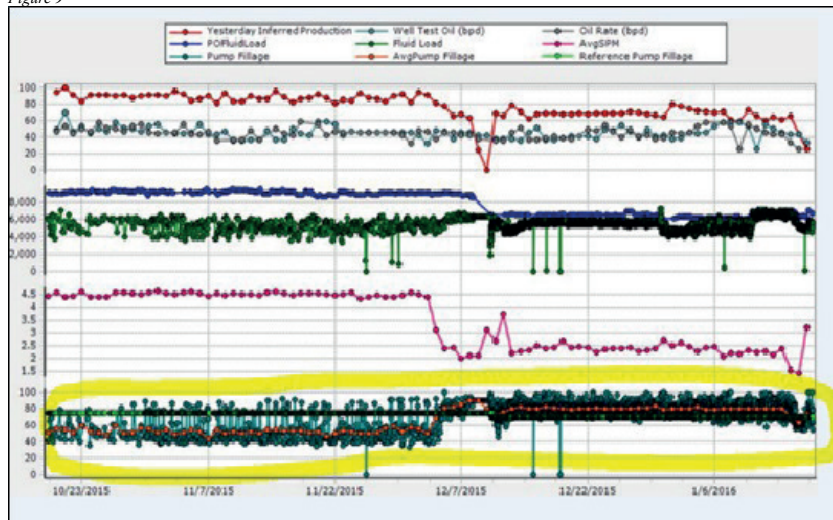
Rod Pump Controller autonomously reduces SPM (reduces speed on downstroke) to maximize pump fillage
