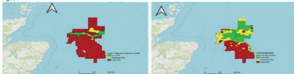
CS reservoir potential for Andrew member (left) and Captain sandstone member (right). Green represents area of low CS risk, yellow represents area of medium CS risk and red represents area of high CS risk.
