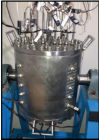
Figure 2. Cylindrical high pressure cell used for hydrate formation experiments
