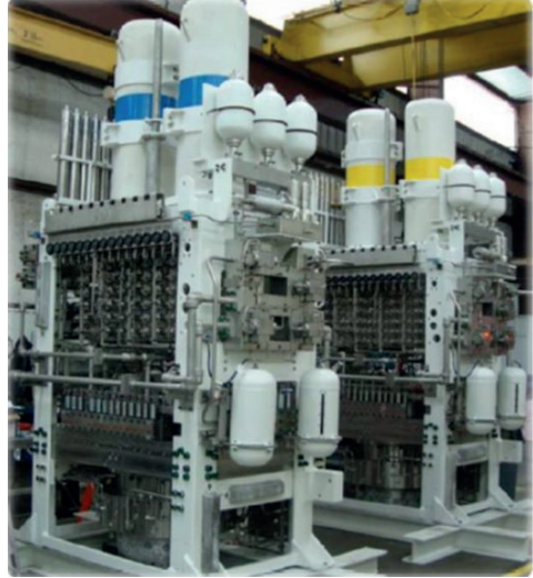
Figure 05 Blue and Yellow Pods - The National Oilwell Varco (NOV) 18 3-4in, 15,000 psi Shaffer
