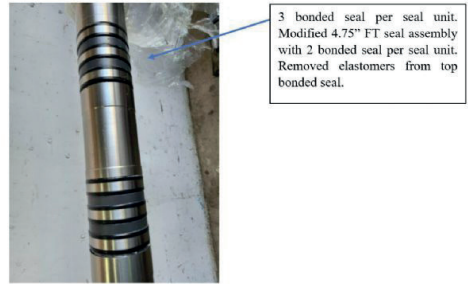
Figure 07 Seal Units- Remove Elastomer from top bonded seal from each seal unit- In Total: 17 Seal Units
