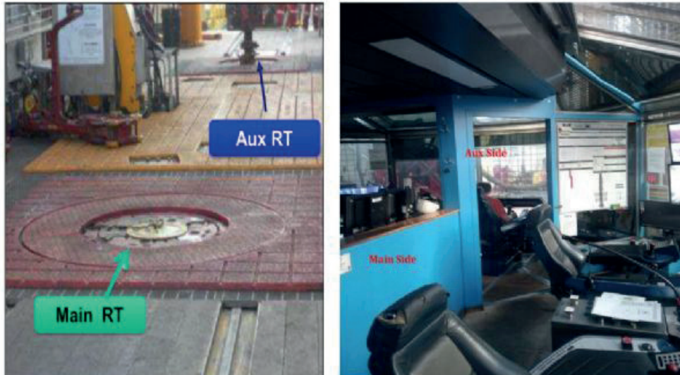
Figure 3 — Main & Aux Rotary Table and Driller's Cabin
