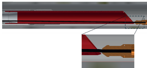
Figure 12: Illustration of how the cable head of the logging toolstring (in gold) can catch on the entry guide of the upper completion (in red).
