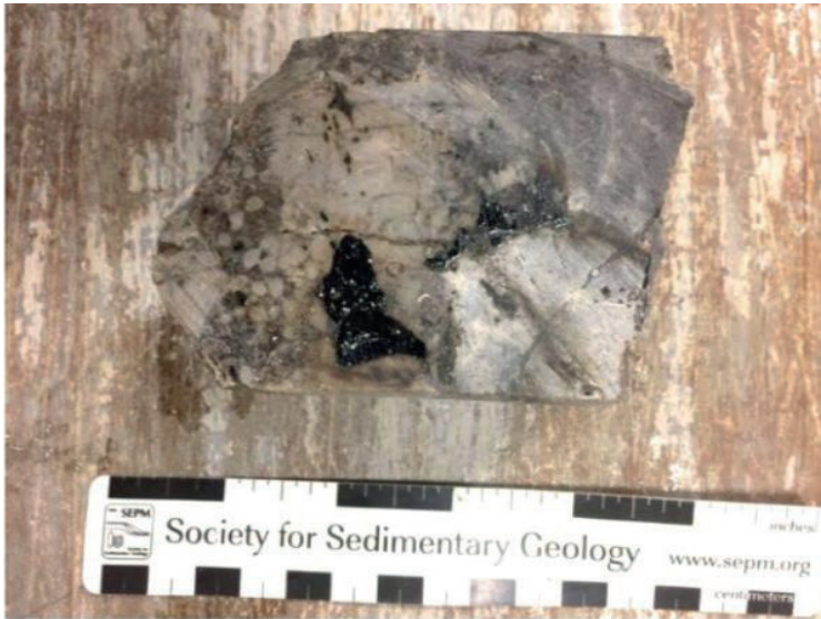
Vuggy Porosity Filled with Hydrocarbon on Cakilli-3 Core (TPAO AR-GEM taken by Ugurlu, I.O, 2017)
