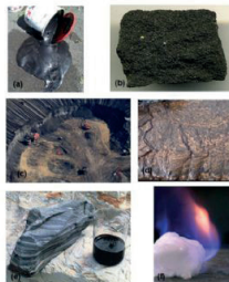
Fig. 3. Unconventional hydrocarbons: (a) Heavy oil not flowing easily due to its high viscosity; (b) A tar sand sample in which bitumen and asphalt fill the pores; (c) An open tar sand mining pit in Alberta; (d) A laminated oil shale sample and lab-
