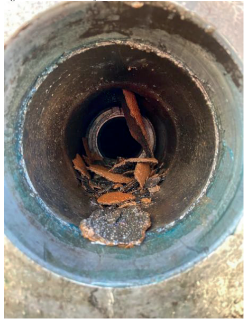
Figure 03-Scale in WT Kit after Well-5- ADJ Box - STX1 condition
